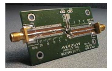
Objective: To provide an optimized solution for a GPS LNA using the MAX2641.
